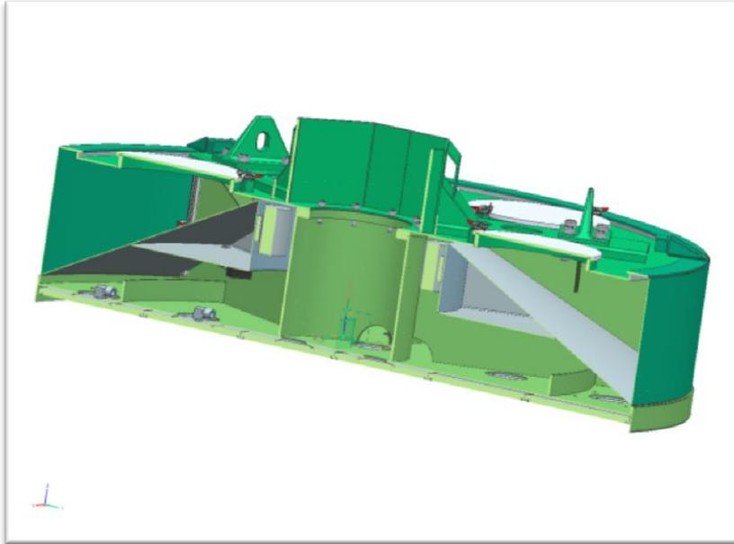
Picture 5. Design for the gripper which includes gap filling compartments.
